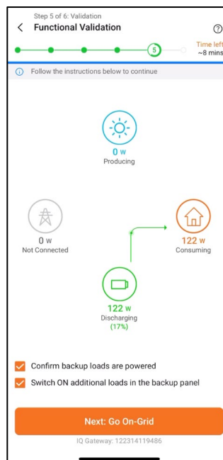
Confirm if backup loads are powered up
